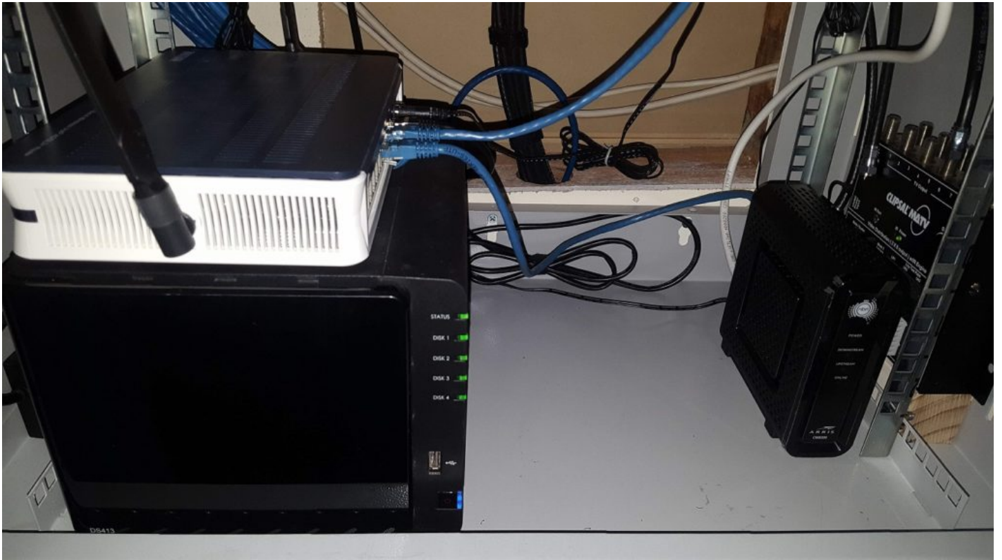
Photo 5: Bottom of cabinet with the old power boards removed, thereby freeing up some space. You can see the Synology NAS on the left with the Billion Router on top and the Arris NBN modem to the right.
