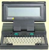
the Osborne, with a case the size of a sewing machine, as mobile).The notebook's hinged design (like a book) consisted of a computer mainboard/keyboard as one half, with a screen on the other half (facing the keyboard).
