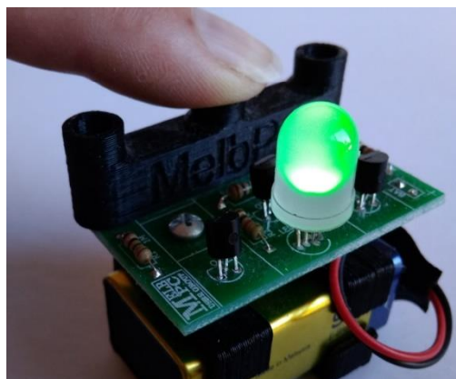
The light Theremin lights up Red, Green or Blue, depending of which of the three light sensors you cover. It will also mix colours.
