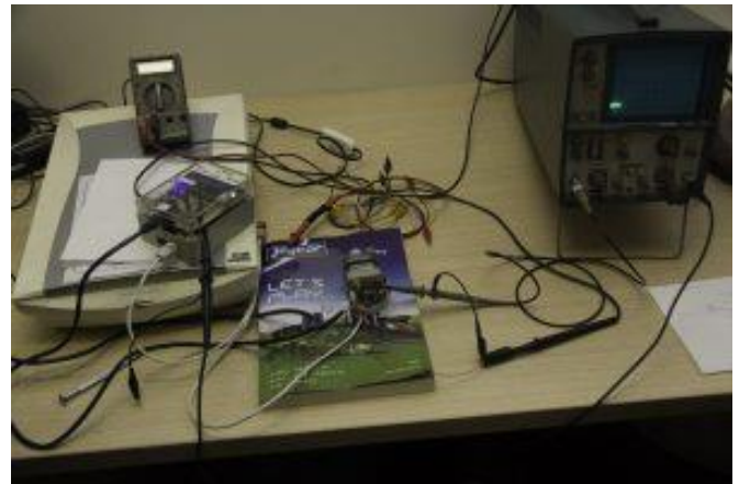
The Microcontroller SIG has a range of electronics test instruments and tools for members' use. The oscilloscope (to the right) is the simpler one of two "CROs" we own and was a valuable debugging tool for John's stepper motor drivers.
