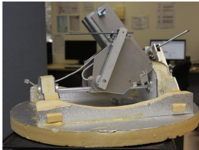
The mirror is steerable in 2 axes, each driven by a stepper motor and lead screw arrangement. John has the mechanical design and machine shop skills to make such a mechanism. The mirror base and support parts are made of lightweight foam, while the reflective surface is metalised Mylar.
