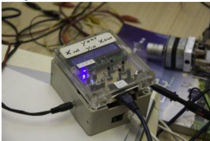
A Raspberry pi B+ in a weatherproof enclosure drives the stepper motors. The stepper motors and drivers are similar to what you'd put in your homebrew 3D printer
