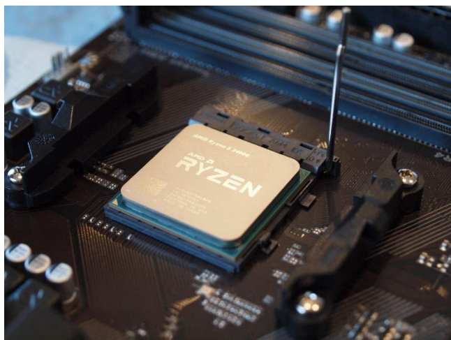
CPU seated in socket, not locked in
