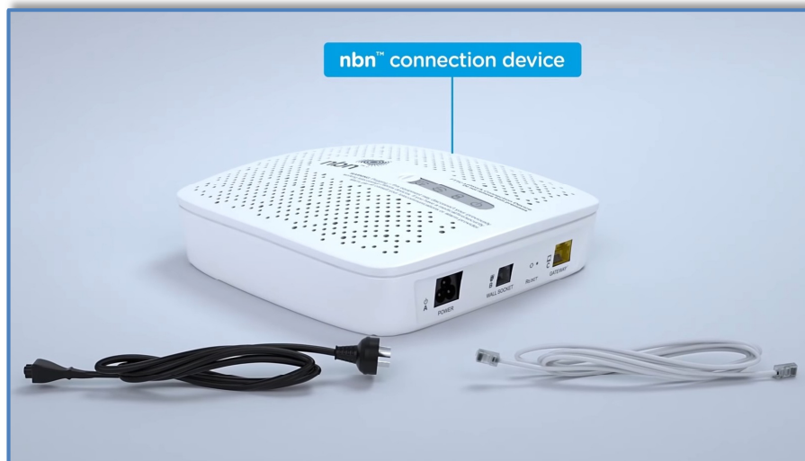
Figure 5 - NBN FTTC Connection Box and cables
