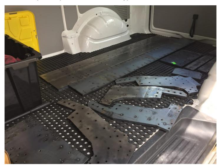
The laser cutting worked rather well, it's quite a clean-cut edge compared to the plasma cutting that I was initially considering.
