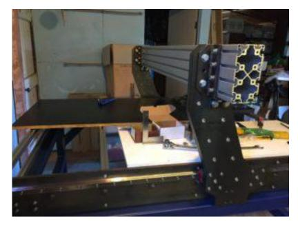
It will all be driven by some closed-loop stepper motors with a decent amount of torque (9 & 12NM), because the gantry is rather heavy with all that steel. The spindle is a 2.2KW water cooled model and should be variable speed control via the software / g-code.
